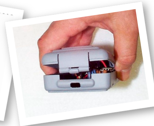
Door Chime hand made model with consumer battery access cover snaps modeled
